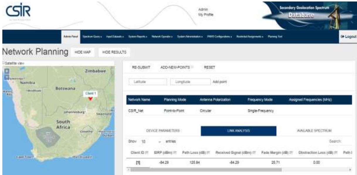
The screenshot displays the CSIR Net-Plan Tool interface. On the left, a map of South Africa is shown with a red triangle indicating a location labeled 'Client 1'. The right side of the interface contains a control panel with buttons for 'RE-SUBMIT', 'ADD-NEW-POINTS', and 'RESET'. Below these are input fields for 'Latitude' and 'Longitude' with an 'Add point' button. A table displays network planning parameters and results:
